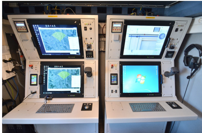
Two-console type GCSs installed in a shelter that can fit on a trailer or in a vehicle mounted housing
