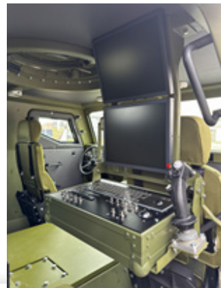
Cabin GCS can be mounted on an army vehicle, such as Alexander and Milosh
