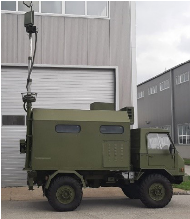
Shelter with GCS and antenna system
