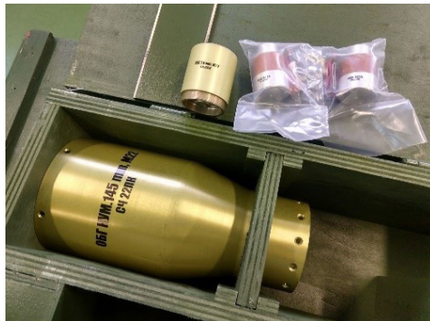
Armor piercing tandem charge WH, 145 mm, 6.4 kg mass, and a spare set of 1 WH TSCWH and 2 fuses
