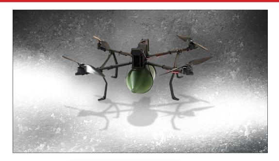
Commercially available drones for single use armed with KPBG 50 anti-armored shape charge - fragmentation warhead of 90 mm caliber. They are intended for actions against armored vehicles, lightly fortified targets and manpower. The system is guided manually toward the target via station or camera control. The warhead is activated by target impact or it may be directed via control station in the appropriate moment.
