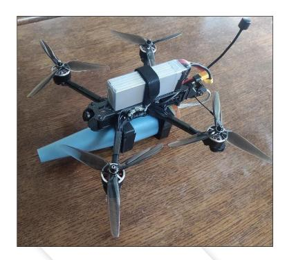
Commercially available drones for single use armed with KPBG 50 anti-armored cumulative fragmentation warhead of 50 mm caliber. They are intended for actions against armored vehicles, lightly fortified targets and manpower. The system is guided manually toward the target via station or camera control. The warhead is activated by target impact or it may be directed via control station in the appropriate moment.
