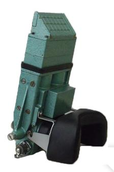
Periscope TVN-2 MS is optoelectronic passive device, that driver of a combat vehicle uses for observation during night and when visibility is very low.
