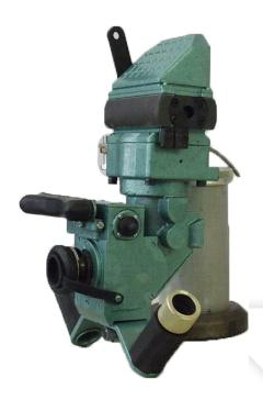
Periscope TKN-1 MS is optoelectronic passive device, that commander of combat vehicle uses for observation during night and when visibility is very low.
