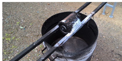
Figure 2 - Details of the fast cook-off resistance testing of the MPE filled payload
