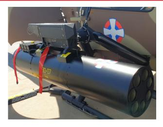
The seven-tube launcher L-80-07 performs individual launches of unguided rockets S-8KOM 80 mm from a helicopter equipped with a "single-channel" electrical installation and devices for launching unguided rockets.
