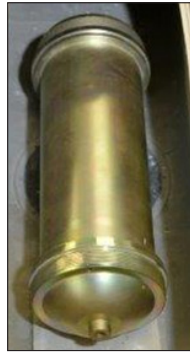
Combined (blast & fragmented), with steel balls, 122 mm, total mass 13 kg
