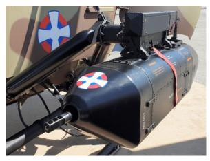
Helicopter pod GH-12.7M with 12,7mm machine-gun is intended for neutralizing ground targets (command posts, light armored vehicles, logistics trucks and enemy's personnel) as well as for fighting against specific air targets (helicopters, light airplanes, RPV-s and parachutists) at effective ranges of up to 1500 m.
