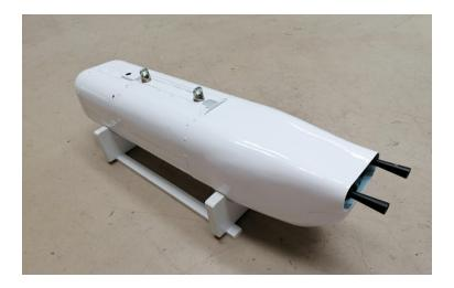
Gun pod GA-2x7,62 mm integrates two machine guns PKT 7.62x54.
