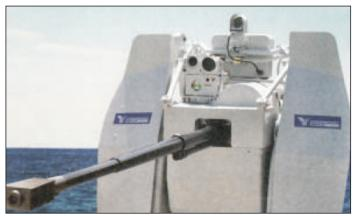
ES LRD-20/M is eye safe, long distance, laser rangefinder module. This module is used in many applications, from demanding military systems to portable devices. Rangefinder operation is based on laser pulse Time-of-Flight (TOF) and is designed to operate reliable under various environmental conditions. This robust device can measure distances up to 20 km.
