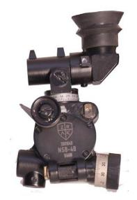
A sighting device NSB-4B is an optomechanical sight, that serves for taking firing elements on elevation and azimuth during direct, semi-indirect and indirect aiming from light mortars 120 mm caliber. It successfully directs mortar in direction of target in daylight and night conditions.
