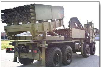
The basic option uses disposable launch pods. The 122/262 mm MLRS is capable of receiving two spare 122 mm launch pods. The system is (un)loaded with a hoisting device mounted on the platform. Another option is to use disposable launch tubes.
