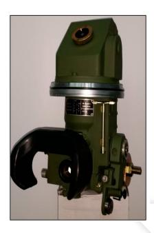
Periscope TPN-1 MS is optoelectronic passive device for T55, that gunner of a combat vehicle uses for observation and firing during night and when visibility is very low.
