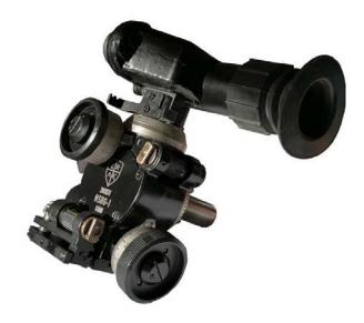
A sighting device NSBG-1 is an optomechanical sight, that serves for taking firing elements on elevation and azimuth during direct, semi-indirect and indirect aiming from Automatic Grenade Launcher 30mm caliber. It successfully aims in daylight conditions and low visibility at night. Indirect aiming and aiming at night is possible on illuminated stationary targets or on targets on move.
