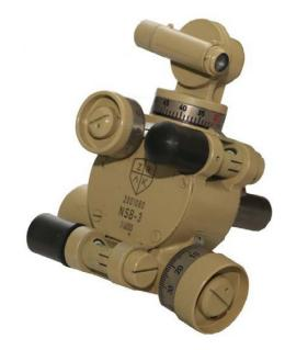
A sighting device NSB-3 is an optomechanical sight, that serves for taking firing elements on elevation and azimuth during direct, semi-indirect and indirect aiming from mortars up to 82mm caliber. It successfully directs mortar in direction of target in daylight and night conditions.
