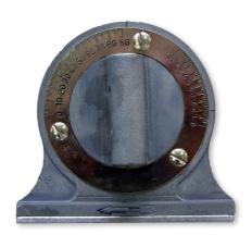
Quadrant set comprises: quadrant, leather case and spare level. Quadrant serves for taking of barrel elevation when sighting device is defective, or for sighting device verification.
