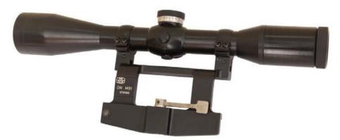
Opto-mechanical sight ON-M91 serves for direct fire, on stationary or moving targets, from 7.62 mm caliber semi-automatic rifle. It successfully aims in daylight conditions, and low visibility at night on the illuminated targets. Mounting sight on weapon can be achieved both with picatinny rail or side mounted (dovetail type).
