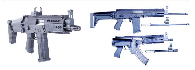
Modular combat system ( MCS ) M19 in calibers 6.5 x 39 mm and 7.62 x 39 mm is gas operated weapon. Main feature of this rifle is easy change of caliber, done by simply replacing the barrel, without disassembling the rifle. Barrels with different lengths, within one caliber, are also available and in that way rifle can be adjusted to different combat situations.
