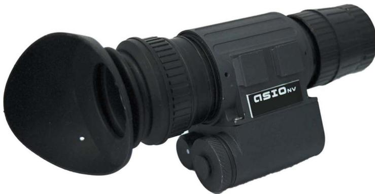
ASIO NV is a night vision multi-purpose monocular. Lightweight and compact, it is intended for observation, surveillance, navigation, or to be used as short to medium ranges weapon sight. ASIO NV utilizes high performance image intensifier tube with integrated power supply, which provides Automatic Brightness Control (ABC) and Bright Source Protection (BSP) to guard against exposure to high levels of light. ASIO NV can be hand-held or worn on a head-mask/helmet for hands-free use.
