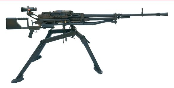
Machine Gun M02 Coyote is formed when the Machine Gun M87 is set to the cradle fixed to a tripod. Pistol triggermechanism and stock with buffer are assembled to the machine gun. These assemblies provide high mobility of the gun, with excellent control of fire.
