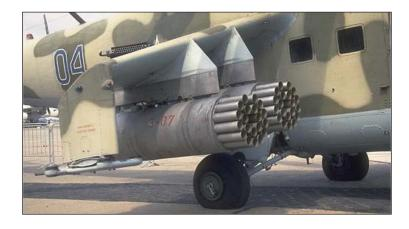
B8V20 rocket launcher is designed to deliver to the designated area and to fire against ground targets caliber 80 mm unguided airborne rockets of various modifications. The B8V20 cluster units are part of the armament of helicopters Mi-8/ Mi-17, Mi-24/ Mi-35, Mi-28H, Ka-31, Ka-52 and their modifications. The cluster unit affords firing of rockets in singles or ripples, depending of the control system used by the currier.
