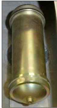
Combined (blast & fragmented), with steel balls, 122 mm, total mass 13 kg
