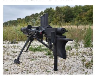
Upgrading of the 20 mm anti-aircraft gun with new solutions to maximally reduce the recoil when firing, made it possible for the rifle to be fired from the shoulder of the shooter, thus obtaining a very efficient large-caliber long-range rifle. The reduction of recoil, vibrations and the shock wave of the powder gases as well as the efficiency of the large-caliber rifle has been achieved with the installation of the following innovative assemblies:
