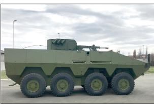
**Lazar 3M infantry fighting vehicle** is equipped with RCWS 30 mm 32V01. It is designed for engagement of enemy personnel (wearing individual body armor), firing assets and unarmored/ lightly armored equipment; reconnaissance and target recognition, surveillance over the environment.
